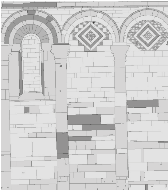
Figure 6 - Detail of the ashlar CAD-map of the first storey (Legenda - yellow: Monte Pisano marble, pale blue: Apuan marble, reddish violet: Eastern marbles, green: serpentinite, pink: red limestone, violet: black limestone, red: replacement stone).
