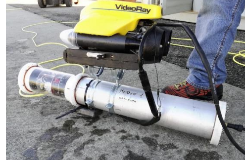
Fig. 11 UOWC modem equipped under the ROV for mobile transmission.
