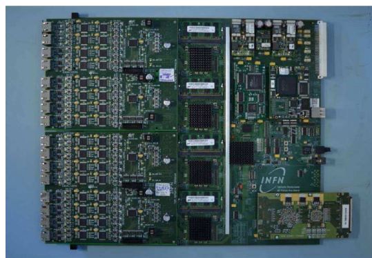
Fig. 15. A TEL62 mounting two TELDES boards.
