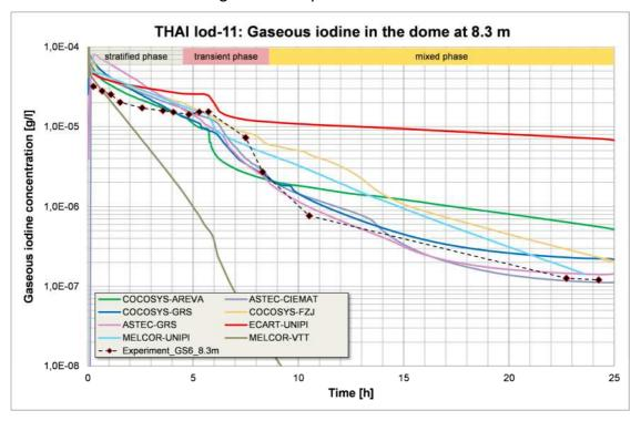
Figure 8: Gaseous iodine evolution along time (data and estimates) - Test THAI lod11
