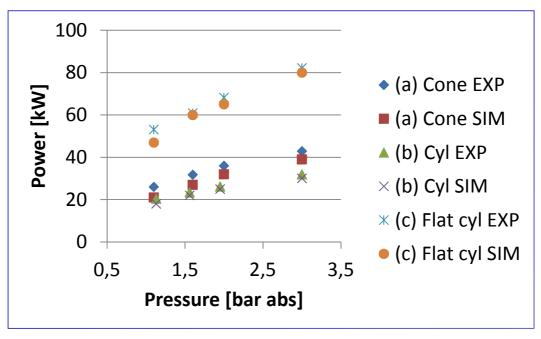
Figure 2: MEWA numerical simulation of the dry-out power for conical and cylindrical shapes of a debris bed in the COOLOCE experiments
