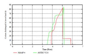
Figure 11: ASTEC-MAAP benchmark on a PWR 900 LFW scenario - In-vessel hydrogen production (left), corium mass in vessel lower head (right)
