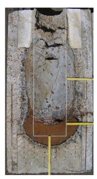
Figure 4: MOCKA Experiments showing post-test cut views with initial cavity positions (left: test without rebars; right: test with rebars)
