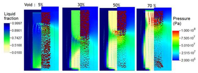
Figure 5: Visualization of flow in 2D calculations with MC3D code. Each picture represents a configuration at a given time for 4 initial void fractions (left part: liquid fraction and velocities (arrows); right part: pressure and gas velocities (arrows); points represent melt fraction)
