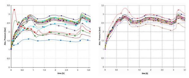
Figure 6: Generic containment benchmark - Pressure in containment dome (the different curves show results obtained by different participants or different codes) - Left: "blind" calculations - Right: "open" calculations
