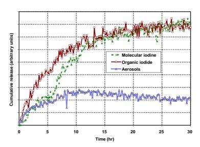
Figure 7: Gaseous iodine production from an iodine loaded painted coupon in EPICUR experiment
