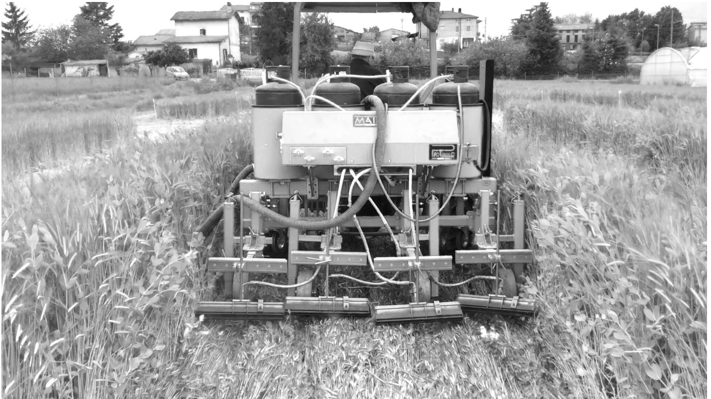
Fig 6. The flaming machine conducting cover crop mixture termination after the roller crimper operation.
