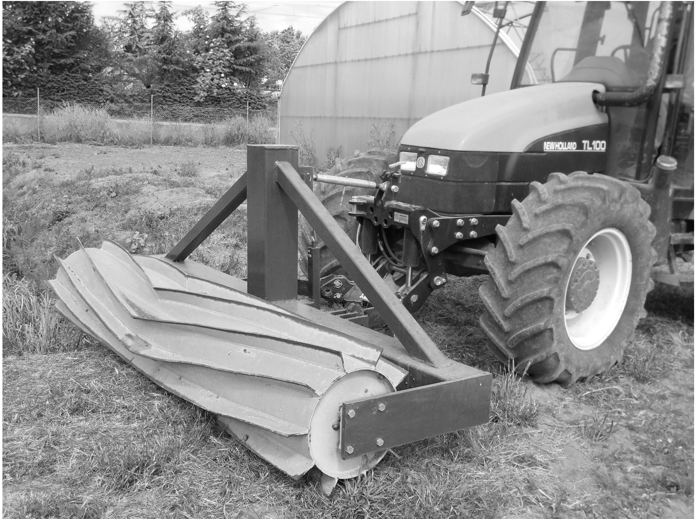
Fig 5. The Rodale Institute design-based roller crimper front-mounted at the New Holland TL100 tractor.
