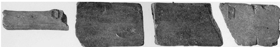
Fig. 1 Testing the alum-treatment on an object where the four pieces fit together, ca. 1905. The right piece was alum-treated. The two pieces in the centre were waterlogged. The left piece was the result of air-drying [6]
