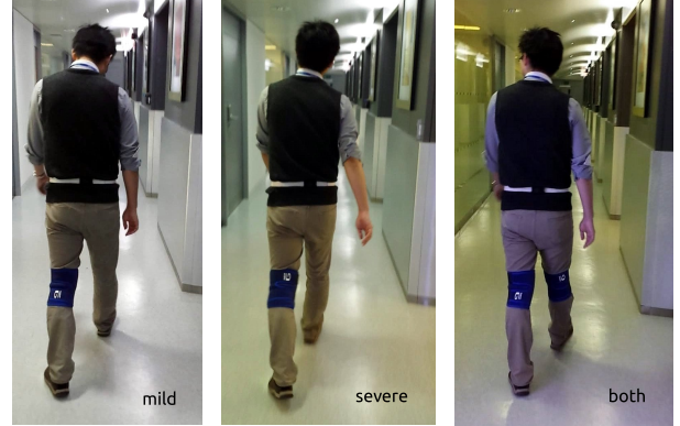
Fig. 2. Each volunteer simulated three different types of impaired gait: mild knee condition, severe knee condition, and mild condition in both knees. Mild condition was simulated using a Neo-G thigh support strap wrapped around one knee. Severe condition was simulated wrapping two straps at the same knee. Finally, to simulate mild problems in both knees, a strap was wrapped around each knee.
