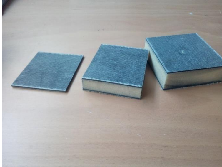
Fig. 1 Samples of the three specimens adopted for the experimental tests: “Skin” on the left side; “Type A” in the middle and “Type B” on the right side.
