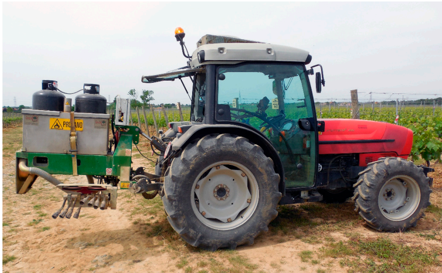
Figure 2. The flaming machine PFV-600 (Officine Mingozi, Ferrara, Italy) coupled with a SAME Frutteto 100 (SAME, Treviso, Italy) tractor.
