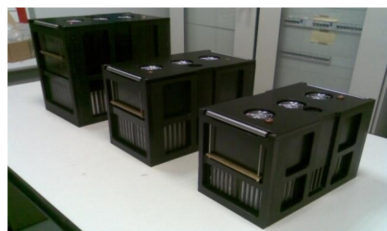
Figure 20: Standard modules: 100 Ah (left), 60 Ah (medium) and 30 Ah (right)
