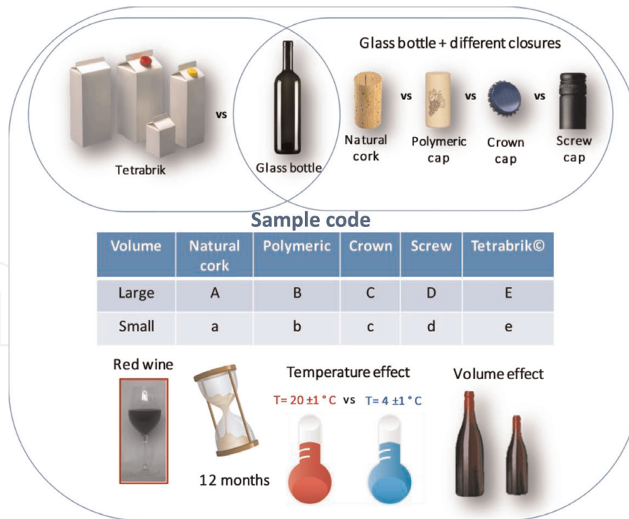
Figure 1. Cases of study 1a, 1b, and 1c: graphical abstract—Experimental setup.
