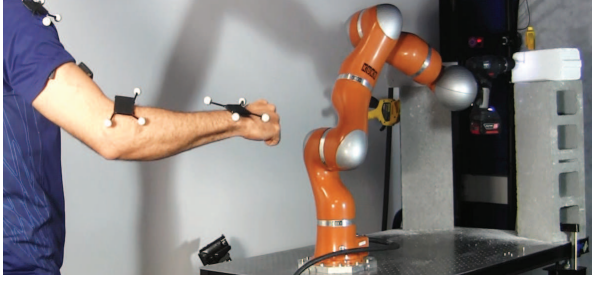
Fig. 1. Experimental setup for remote drilling of hard objects (bricks) in different positions and orientations of the robot workspace. To accomplish the task, the operator must adjust the endpoint stiffness profile of the robot end-effector to achieve the task-required interaction force profile in different phases of the task.
