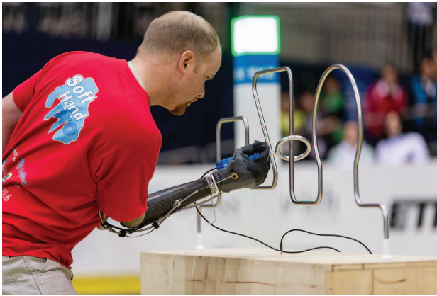
Figure 1. The SHPH and our pilot (SoftHand Pro team) performing the wire-loop task at C-PAPR. (Photo courtesy of ETH Zürich.)
