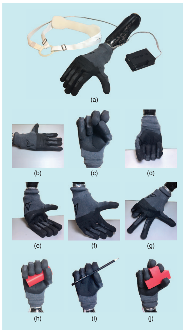
Figure 4. (a) The SHPH prototype adopted for the C-PAPR and its main components: the hand, the socket, the body power harness, and the battery pack. The main hand postures available to the user include (b) flat hand, (c) grasp closure, (d) and fist. (e)–(g) The soft behavior of the SoftHand and its robustness in several interactions with the environment. (h)–(j) The main grasping capabilities of the hand, highlighting the intrinsic adaptability to object shape.
