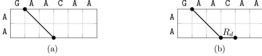
Figure 4: (4a) diagonal j = 1 : lce_{S,P}(0, 1) = 2 , thus the 0-FRP reaches the last row of the table and k_E -EXT correctly returns pair (2, 0) . (4b) diagonal j+d = 2 : R_d(|S|, |P|, ST_{P,S}^*, 1, 2) returns (r_d, c_d) = (1, 3) (as lce_{S,P}(2, 4) = 0 ): since r_d = |S| - 1 , this path reaches the last row of the DP table, and k_E -EXT correctly returns pair (3, 1) .
