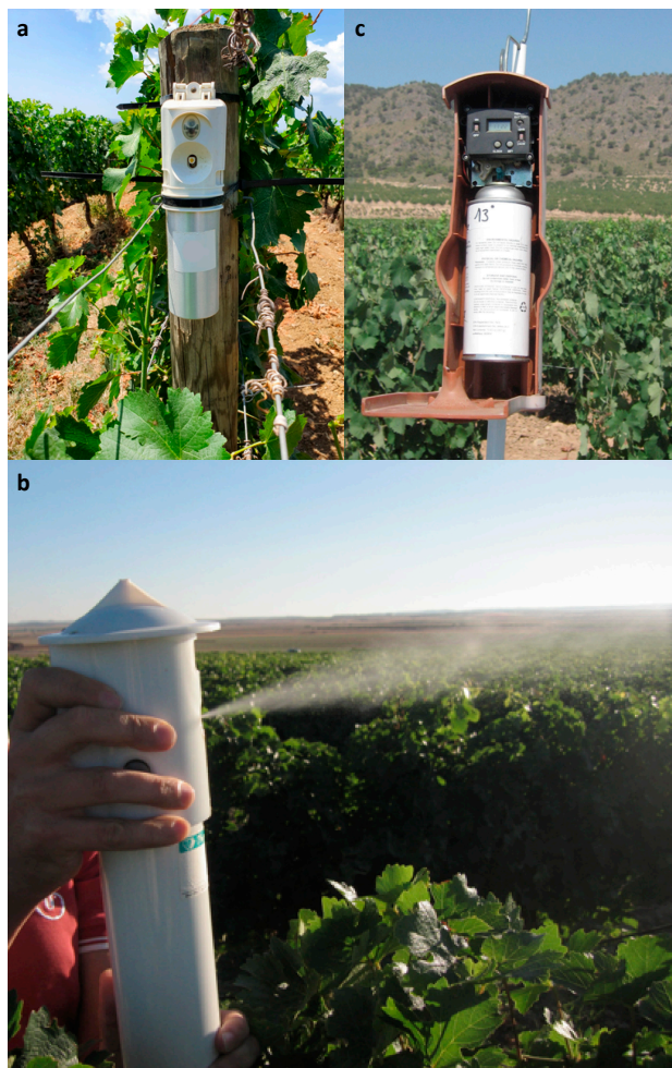
Figure 3. Aerosol devices used for pheromone-mediated mating disruption of the European grapevine moth, Lobesia botrana , on grapevine: (a) Isonet® MISTER PRO L, (b) Isonet® MISTER releasing a puff of L. botrana pheromone in a Spanish vineyard, (c) CheckMate® Puffer® LB (Sutterra) (photo credit: Andrea Lucchi).
