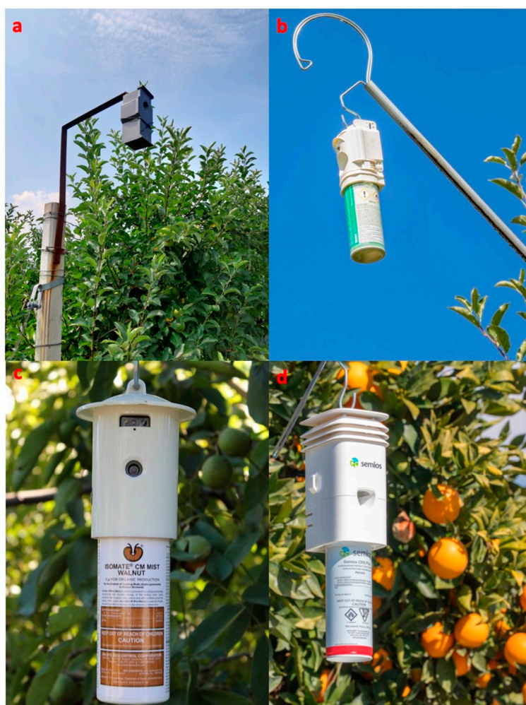
Figure 1. Examples of aerosol devices currently marketed (2018) for pheromone-mediated mating disruption of the codling moth, Cydia pomonella , in apple orchards, (a) CHECKMATE Puffer® CM (Suterra), (b) ISOMATE® CM MISTER (CBC Europe Srl-Italy) (photo credit: Claudio Ioriatti), (c) and in walnut orchards, ISOMATE® CM MIST WALNUT (photo credit: Tina Phelps). (d) Management of Aonidiella aurantii in orange groves relying to Semios CRS Plus (Semios Technologies Inc. Canada) (photo credit: Kelly Petersen).
