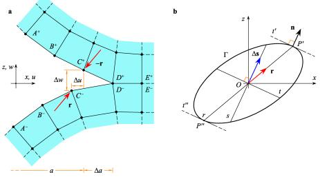
Figure 1: (a) virtual crack closure; (b) ellipse of crack-tip flexibility.
