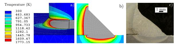
Figure 9. Constant initial temperature: Overview of the thermal solution (a), FE-model cross section of the weld seam (b), and real cross section of the weld seam (c).
