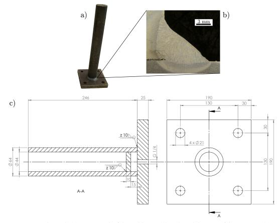
Figure 1. Real sample (a), micrograph of the weld seam (b), technical drawing of the specimen (c).
