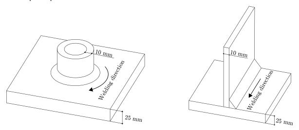
Figure 11. Real specimen's geometry (left), simplified specimen's geometry (right).
