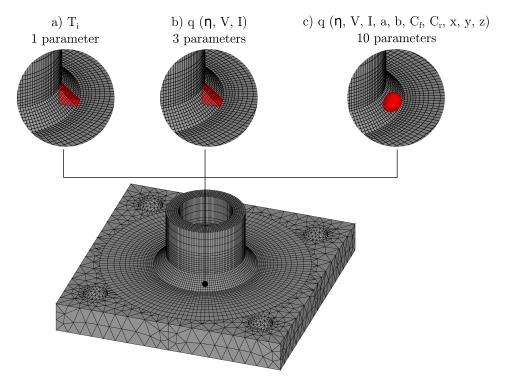
**Figure 3.** Meshed specimen (bottom) and simulation techniques applied on the welding seam: constant initial temperature (**a**), constant heat flux (**b**), and Goldak's double-ellipsoid model (**c**).
