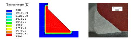
**Figure 4.** Activated elements for the constant initial temperature (CIT) model with a temperature of  $T_i$  (**left**) cross section of the weld seam (**right**).
