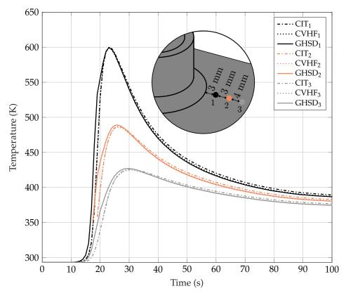
**Figure 14.** Temperature vs. Time curve of the thermal models employed, specifically for three points on the surface of the plate.
