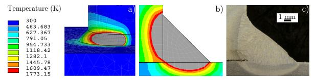
**Figure 7.** Goldak's double-ellipsoid model: Overview of the thermal solution (**a**), finite-element (FE)-model cross section of the weld seam (**b**), real cross section of the weld seam (**c**).
