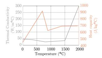
Figure 2. Temperature dependent thermal material properties derived from [20].
