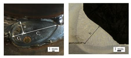
Figure 6. Goldak's heat source parameters obtained directly by the fusion zone.
