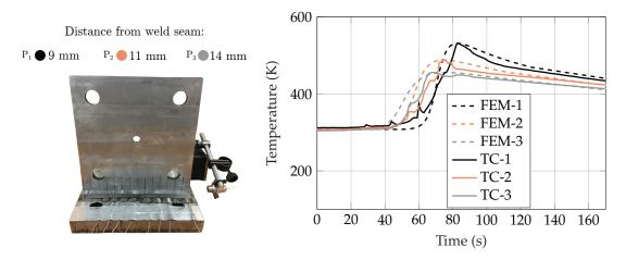
Figure 15. Comparison between experimental and numerical results of temperature over time.
