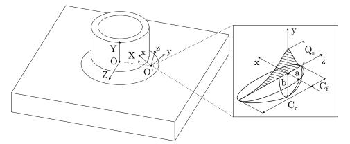
Figure 5. Coordinate system transformation between global and local reference frame, for Goldak's double-ellipsoid model.
