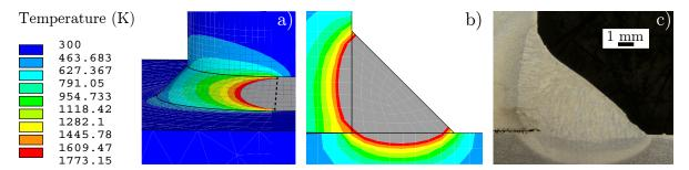
Figure 8. Heat flux model: Overview of the thermal solution (a), FE-model cross section of the weld seam (b), and real cross section of the weld seam (c).
