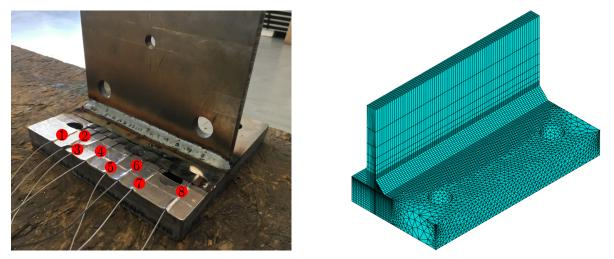
**Figure 10.** Experimental set-up for temperature measurement (**left**) and FE-model (**right**) of the simplified specimen.
