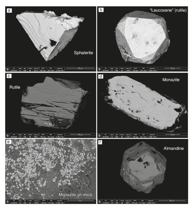
Figure 5. Back-scattered electron images of high-density crystals and crystal fragments extracted from sample #32 (Rio San Pantaleone, Santa Maria del Giudice, Lucca). a) nearly complete tetrahedral crystal of sphalerite; b) equant crystal replaced of "leucoxene"; c) fractured subhedral crystal of rutile; d) subhedral crystal of "monazite"; e) tiny crystals of "monazite" grown on mica; f) euhedral, slightly abraded, dodecahedral crystal of almandine.
