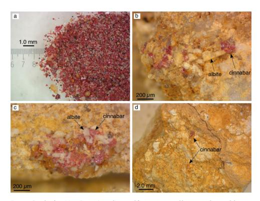
Figure 4. Cinnabar from Monti Pisani. a) cinnabar crystal fragments extracted by panning about ten kilograms of low-temperature hydrothermal material from the small trench in the Monte Zano (Vorno, Lucca) area; b,c,d) crystalline cinnabar *in situ* from the same trench.
