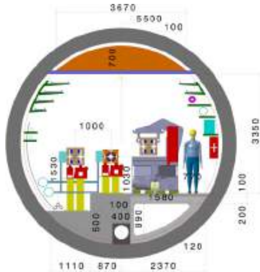
Fig. 6. Machine tunnel cross section in a regular arc with machine elements, services and transport equipment.
