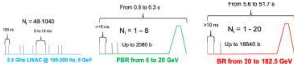
Fig. 6.2. Schematic representation of the FCC-ee injector scheme showing the bunch structures and the magnetic cycles in the PBR and BR (green and red respectively).
