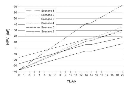
**Figure 4.** Evaluation of MH Floodlights replacement with LED Floodlights: trends of NPV in function of the time (investment by own founds, r = 2%).
