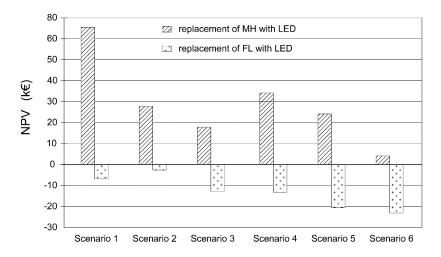
**Figure 5.** NPV values for MH floodlights and FL luminaires replacement with LED floodlight (investment by own founds, r = 2%).
