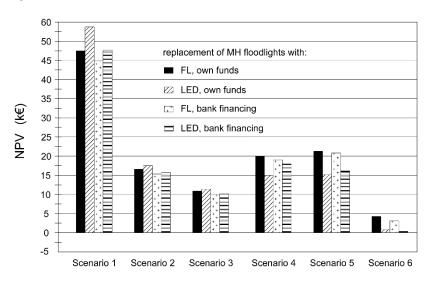
Figure 6. NPV values obtained for different MH floodlights replacement.
