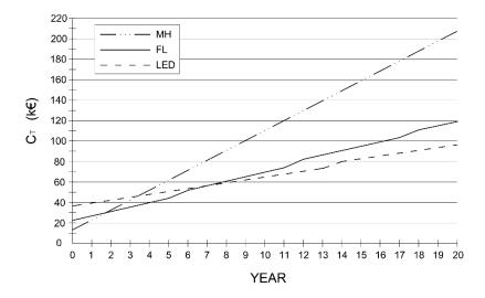
**Figure 2.** Trend of  $C_T$  discounted values in function of time, for lighting systems with different luminaires: results of scenario 1.
