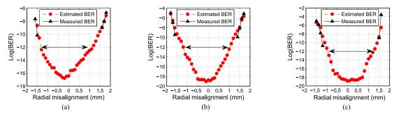
Fig. 3. Tolerance to misalignment: BER vs. radial misalignment for 3 mm (a), 4 mm (b), 5 mm (c) ball lens.
