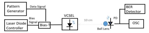
Fig. 1. OWC experimental setup at 2.5 Gb/s and 10 cm distance. OSC: Sampling oscilloscope; PD: PIN photodiode+TIA.
