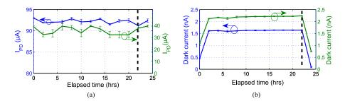
Fig. 10. Received current (a) and dark current (b) of the photodiode with the quartz ball lens as function of time (Xrays dose : 10.8 Mrad/hour).
