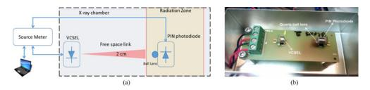
Fig. 7. (a): X-rays irradiation test setup; (b): PCB with the VCSEL and the photodiode with a ball lens.
