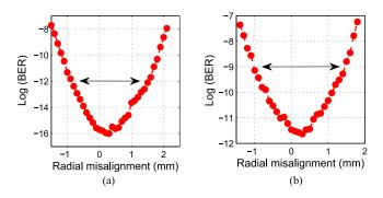
Fig. 4. Estimated BER vs. radial misalignment at 15 cm (a) and 20 cm (b) transmission distance.
