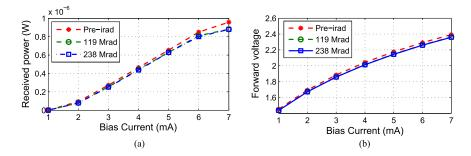
Fig. 8. (a): L-I curve of the VCSEL; (b): I-V curve of the VCSEL under X-rays.
