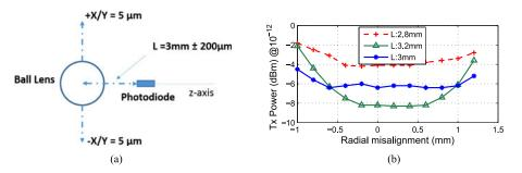
Fig. 5. (a): Scheme of packaging tolerance for the lens; (b): transmitted (Tx) power as a function of radial misalignment considering 5  $\mu$ m deviation on X/Y axis and for different values of L (z-axis).
