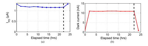
Fig. 9. (a): Received current at the photodiode as a function of time; (b): dark current of the photodiode at a reverse bias of 4 V as a function of time with 10.8 Mrad/hour dose. Bar line shows end of irradiation test.
