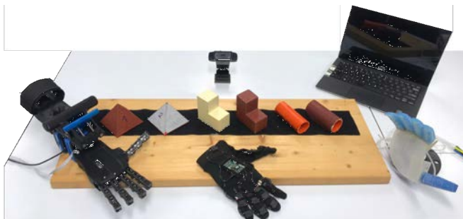
Fig. 5. Experimental Setup used in this paper. Two soft robotic hands (namely RBO Hand and Pisa/IIT SoftHand) were used to grasp six objects with different shape and surface roughness. A camera was used to record the whole experimental execution. Accelerations of the fingers were recorded through a custom glove endowed with 16 IMUs.
