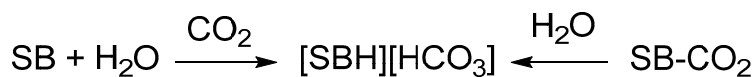
Scheme 7. Formation of bicarbonates by reaction of CO 2 with wet superbases (SB) or by hydrolysis of pre-formed SB-CO 2 adducts.
