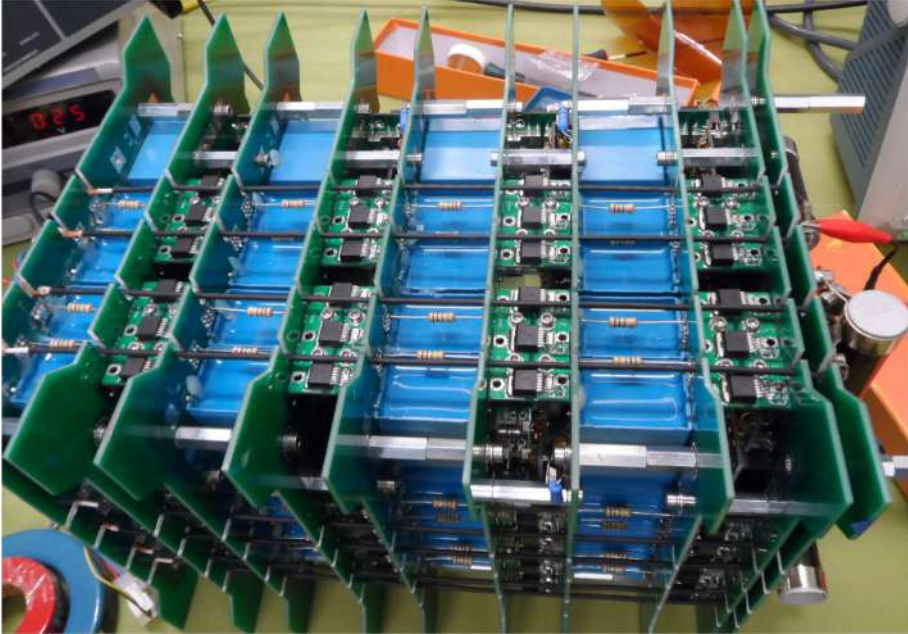
Fig. 3.21. Four stage Marx generator assembled in a coaxial structure (four return conductors per side).
