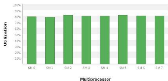
Figure 5: Compute utilization of the streaming multiprocessors on the GTX 680 for the fitting kernel of the two kernel fit implementation.
