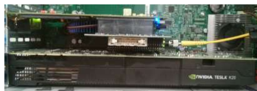
Figure 6: The TTCrq-interface-NaNet system together with a NVIDIA Tesla K20 GPU.
