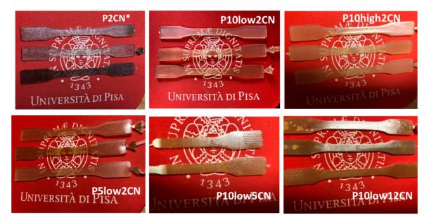
Figure 5. specimens obtained by injection moulding: comparison regarding transparency.
