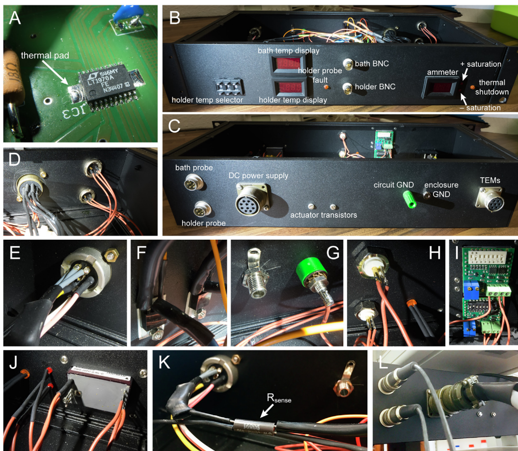
Fig. 4. Backstage enclosure components and essential wiring diagram to the PCB. (A) Closeup on the power actuator chip, which requires soldering a bottom thermal pad. (B) Front plate. (C) Back plate. (D) DC power (left) and temperature probe receptacles (right). (E) TEM connector receptacle. (F) PNP and NPN power actuator transistors use the back plate as heat sink. (G) Enclosure (left) and circuit (right) grounding jacks. (H) Chamber holder and bath temperature output BNCs. (I) Chamber holder and bath temperature displays. (J) Ammeter. (K) Current sensing resistor. (L) Probe and power supply plugs connected to the backstage enclosure.
