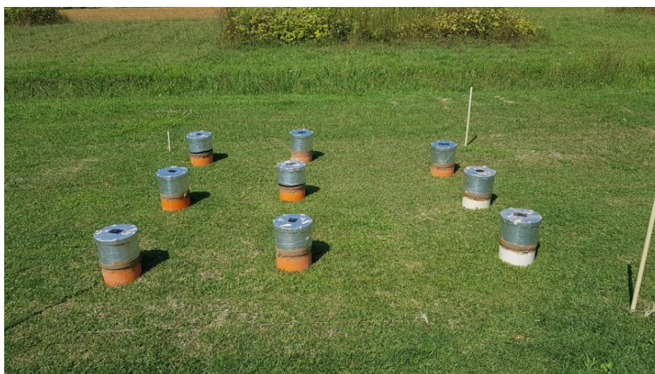
Figure 2. Static chambers for the monitoring of CO 2 and CH 4 emissions by turfgrass
