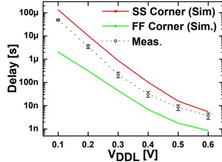
Fig.8. Measured delay versus  $V_{DDL}$ .
