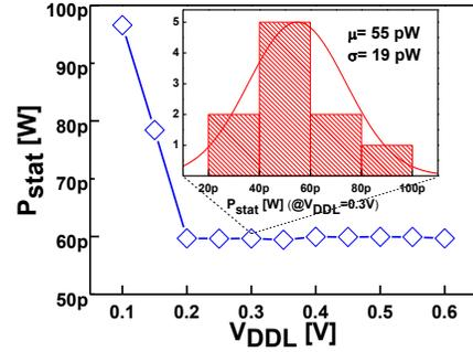
Fig.7. Measured static power versus  $V_{DDL}$ .
