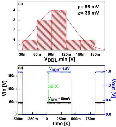
Fig.6.  $V_{DDL,min}$  measurements: a) Distribution of minimum  $V_{DDL}$  for successful up-conversion to 1.8V; b) Measured waveform for a 50mV to 1.8V conversion.
