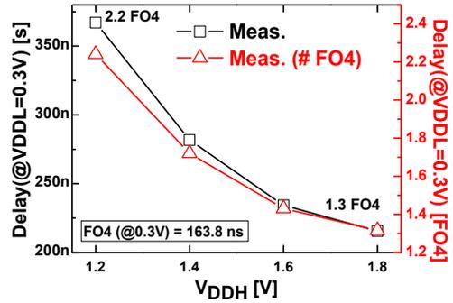
Fig.9. Measured delay versus  $V_{DDH}$ .
