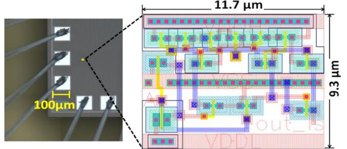
Fig.5. Micrograph of the testing chip and layout of the proposed level shifter.
