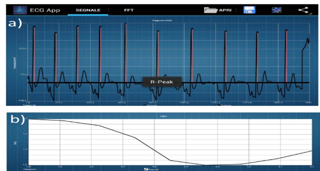
Fig. 4. Example of signals acquired from the wearable system: a) ECG; b) obtained HRV;
