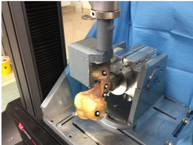
Fig. 3 – FMPC tensile test set up. A specific mechanical frame was designed to align the FMPC specimen with the 5 kN load cell to obtain a correct uniaxial tensile test in anatomical position.
