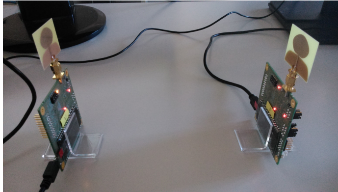
Fig. 19. DecaWave EVB1000 UWB boards used in the real environment.
