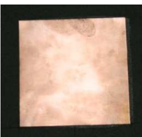
Figure 3d - Copper-foil patch antenna on textile substrate.
