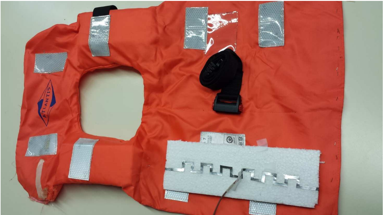
Figure 10: Grounded folded meandered dipoles for integration on the floating elements of a lifejacket, operating at the Cospas-Sarsat 406MHz band. The two-antenna configuration consists of two folded meandered dipoles perpendicularly oriented, one behind the neck and the other one at the front of the chest (or both at the front side) [91].
