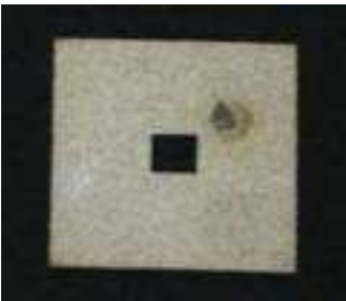
Figure 3c - Screen-printed textile patch antenna.
