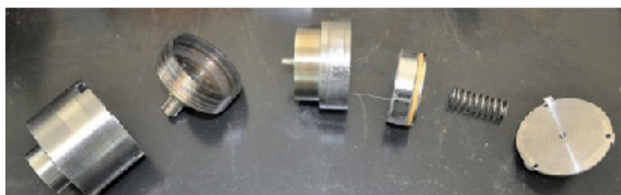
(b) Disassembled prototype: the external case, the multidisc rotor, the internal cylinder, the magnets system with shields and pneumatic o-ring, the spring and the rear cap (rightward order).
