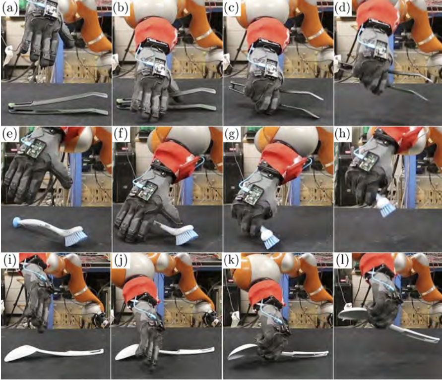
Figure 1.13 Snapshot of pinch grasps generated through the proposed architecture. Subfigs a-d show a pinch grasp performed on object 7; subfigs e-h show a pinch-left grasp performed on object 8; subfigs i-l show a pinch-right grasp performed on object 9. For each line, it is possible to observe an approaching phase (e.g. subfigs a-b), a contact detection (e.g. subfig b), and a firm grasp and lift of the object (e.g. subfig c-d).
