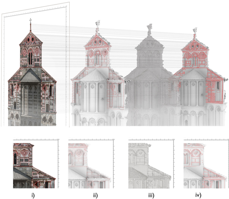
Figure 4. Steps of the proposed methodological approach, involving: i) thematic mapping over the orthophoto; ii) projection of annotations on the mesh representation; iii) point-based representation and iv) point-based thematic mapping over the 3D model.
