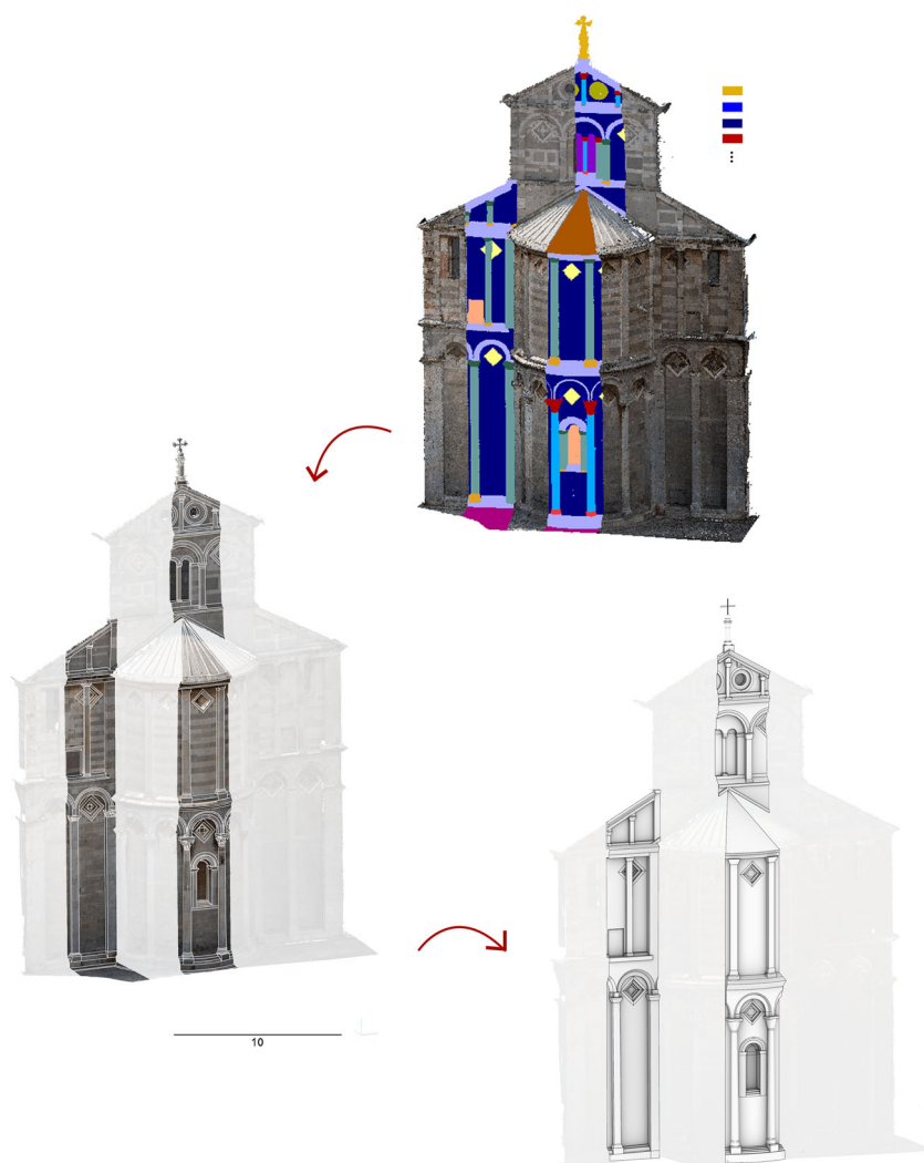
Figure 19. Semantic segmentation of the model with identification of classes of typological elements. Future work will consider the model resampling based on these primitive architectural components.
