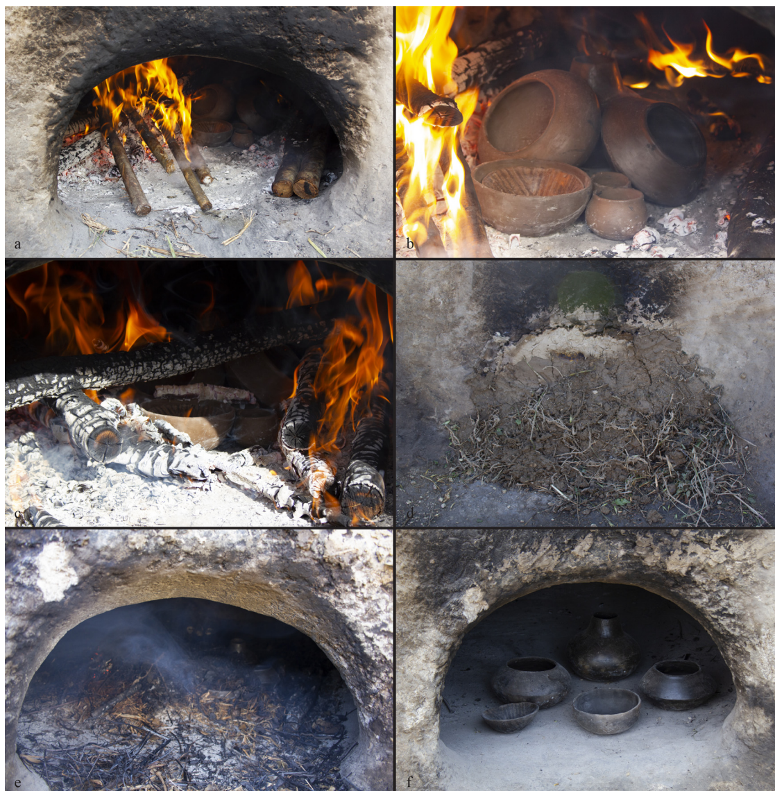
Figure 6: Reducing pottery firing (A). (a and b) Heating step, (c) firing, (d) reduction step plugging the frontal opening with a mixture of clay and straw, (e) opening of the oven after the cooling phase, and (f) final result.
