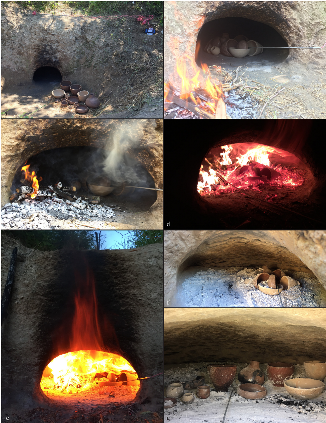
Figure 7: Oxidising pottery firing (B). (a) Preparation of the experiment and setting of the thermocouples, (b and c) heating step, (d and e) firing, (f) state of oven and vessels after the cooling phase, and (g) final result.
