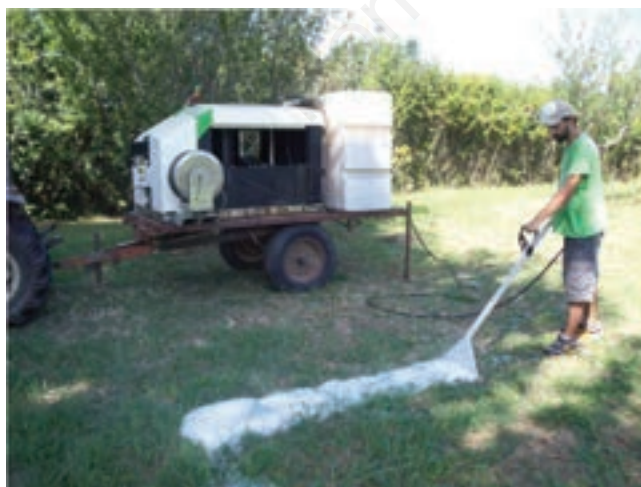
Figure 1. Hot foam machine: operator using the hot foam distribution tool and lateral view of the machine with the 1000 L water container, the covered part containing the foam container, the boiler, the programmable logic controller, the pump and the diesel generator set.
