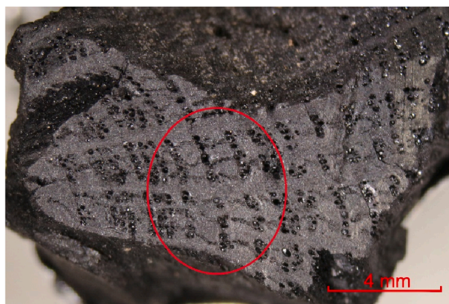
Fig. 12. Sample 6 (USHO17): white oak group; the flame-like arrangements of vessels of latewood. (Photo by B. Gmińska-Nowak).
