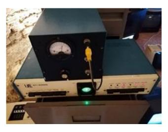
Fig. 10: Modem and power supply for Olivetti teletype
