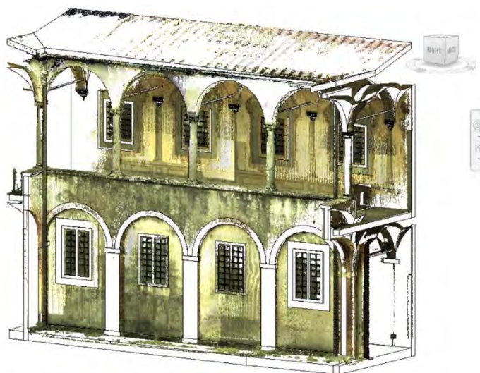
Figure 22. Point cloud displayed over the reconstructed parametric model.
