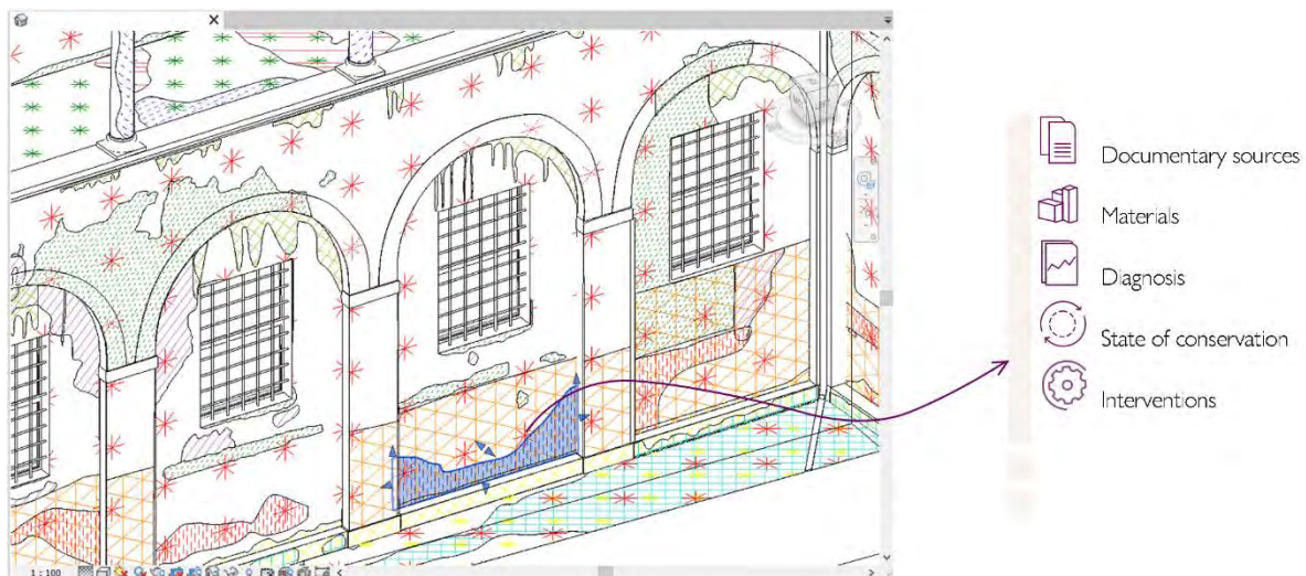
Figure 20. Insertion of further idealized information on the parametric model.
