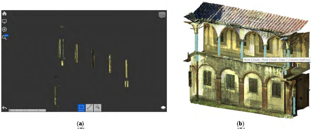
Figure 14. Label 7—Column shaft imported into Recap upfront (a) and later selected on the overall point cloud in Revit (b).
