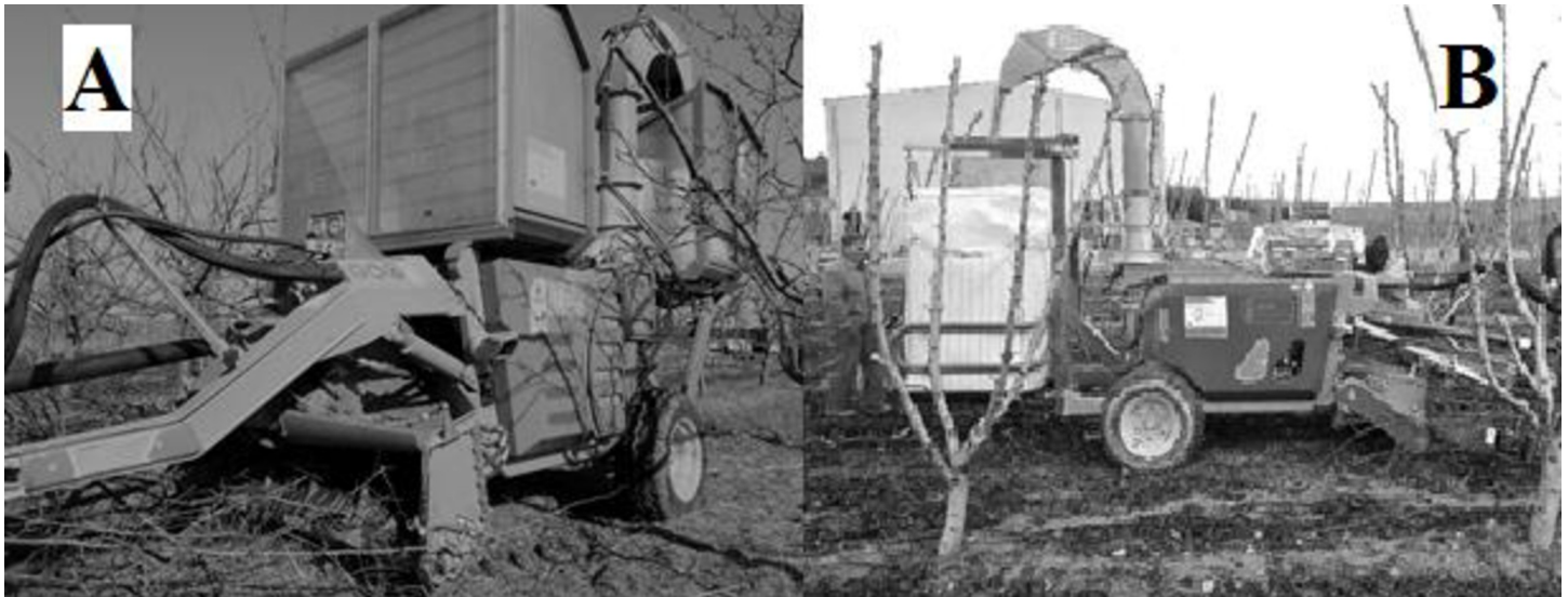
Fig 1. Naldoni prototype PC50 at different configuration. A) tilting box and B) big-bag during the harvesting.
