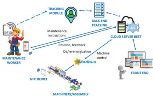
Fig. 1. Main components of the novel smart system for the safe management of the de-energization/re-energization process.
