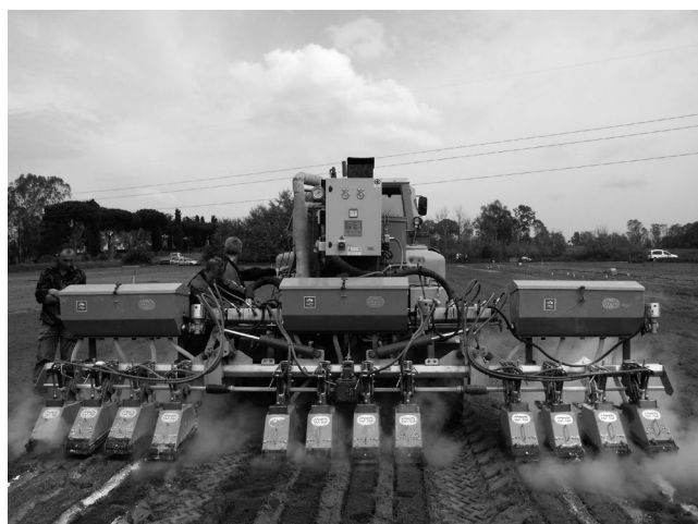
FIGURE 1 Band-steaming machine performing steam application at site I on 4 April 2012
