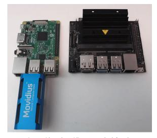
**FIGURE 3.** RPi 3B+ with Intel Movidius NCS on the *left* and NVIDIA Jetson Nano on the *right*.
