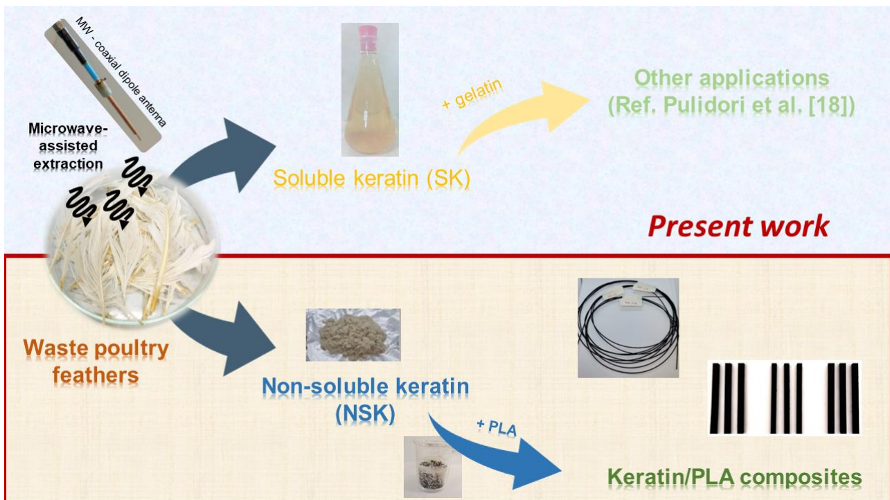
Figure 1. Scheme of the valorization of keratin from waste poultry feathers obtaining soluble keratin and keratin/PLA composites.
