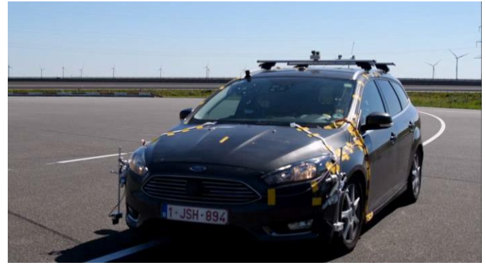
Figure 14. Instrumented vehicle for the 15DOF and tire model identification method proposed in the paper.
