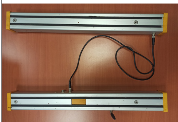
FIGURE 122 Example of an electronic hive scale
