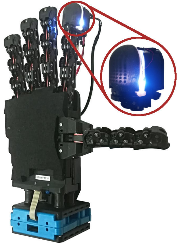
Fig. 1: The QB SoftHand with an integrated neuromorphic optical tactile sensor. The neuroTac is integrated with the hand's index finger.
