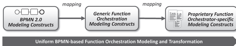
FIGURE 6 An approach for uniform modeling and transformation of function orchestrations using BPMN
